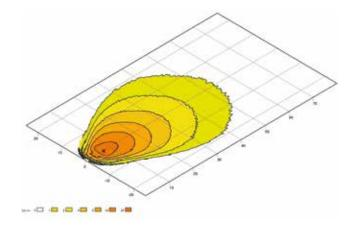
Isolux diagrams are used to compare illumination. The intensity of illumination is measured with an incident light meter to determine if a work area is sufficiently lit up.
