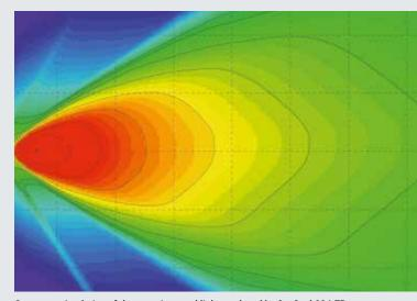
Computer simulation of the superimposed light produced by 2 x Oval 90 LED worklights shows how a harmonious overall pattern is produced.
